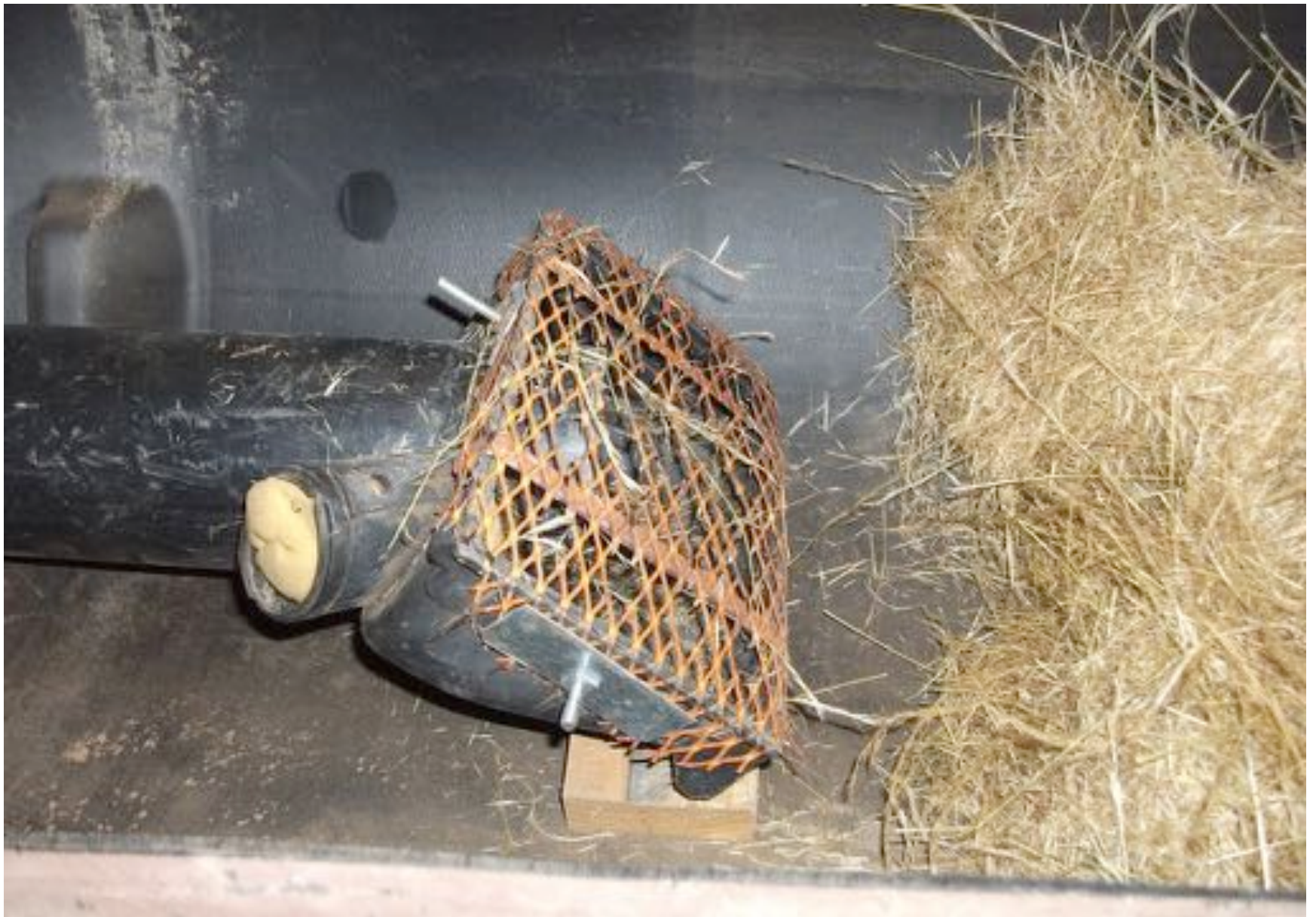
With mesh from an ironing board attached to end of suction pipe inside seed hopper.
