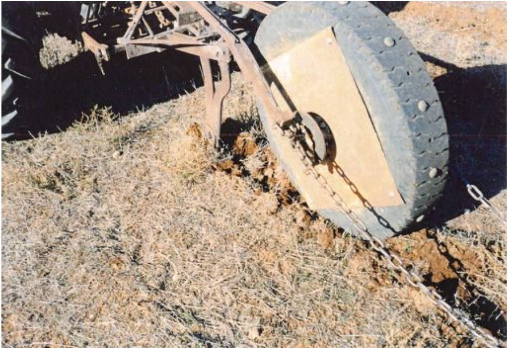
Home-made combination ripper and seed hopper.
