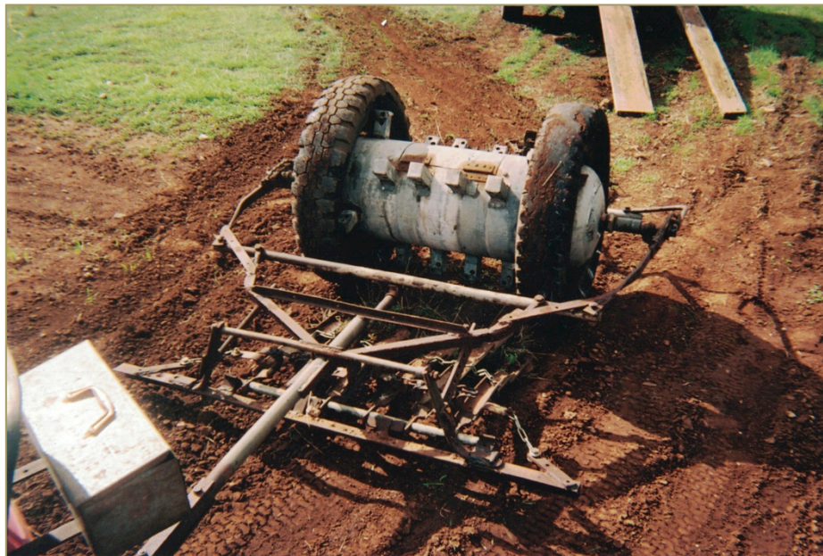
Photo 12: My "six row" seeder made with a large gas bottle fitted between two tyres.
