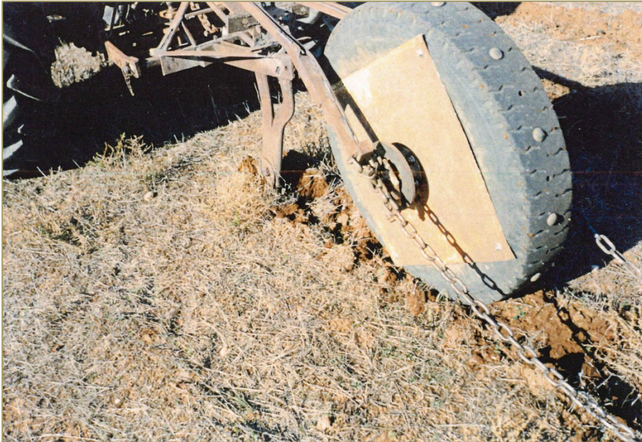
Photo 11: A square metal plate is attached to one side of a truck tyre to form a rolling hopper. Holes are drilled in the outer surface of the tyre to allow seeds to fall through. Some holes are plugged with bolts.
