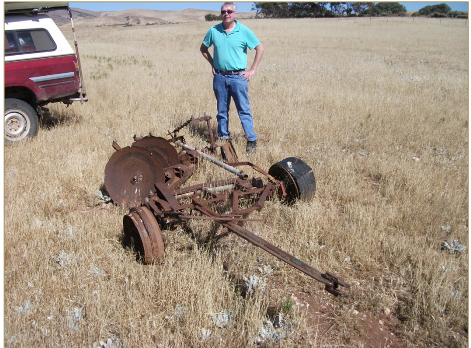
Photo 7: The four-furrow disc plough made from scrap metal towed by my 4WD ute (at left).
