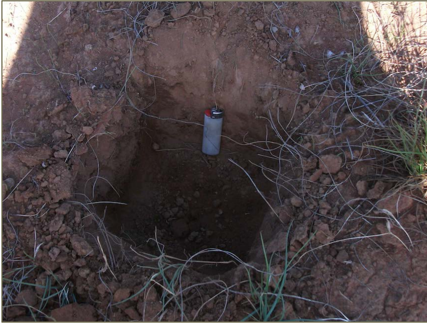
Figure 23: 9th April 2015, three days after a significant rainfall event. A hole dug into cultivated soil reveals moisture penetration to beyond 50cm deep – the depth of the hole. This means that surface salt has been drawn down to at least this depth by rainfall seeping in to the ground. However, note that the top 10-15cm of soil is dry.
