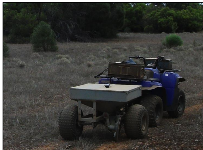
Figure 8: Rabbit bait-layer being towed by quad-cycle. Small plough disc at rear cuts the shallow groove for the baited seed to fall in.
