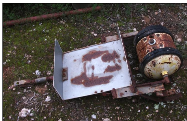
Figure 10: Seed dispensing drum made from an old 4.5 kg barbecue cylinder fitted in an A-frame. Tow point is at the left. Strips of car tyre bolted to outside edge of drum to provide ground clearance for delivery hole. Sheet metal tray fitted for carrying various extra supplies.
