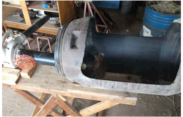
Garden leaf blower (left) with homemade hopper and feed system (right) make distributing Spear Grass seed a "breeze"!
