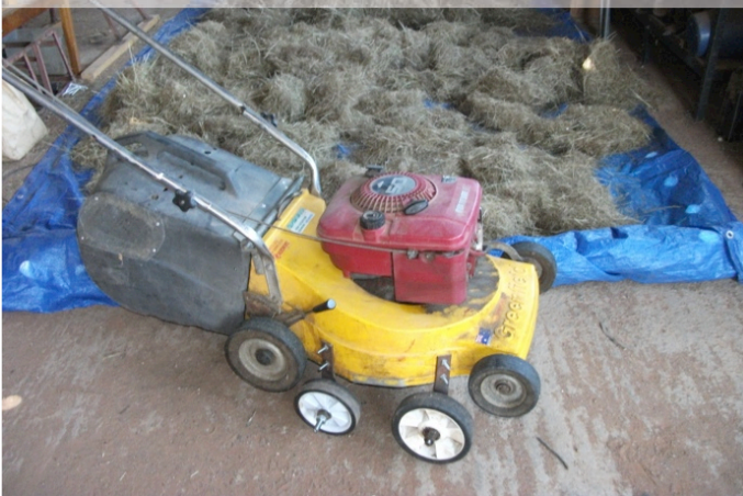
Grass seed harvester made from a lawn mower, on "raised legs". In the background, harvested Spear Grass seed is spread out for drying.
